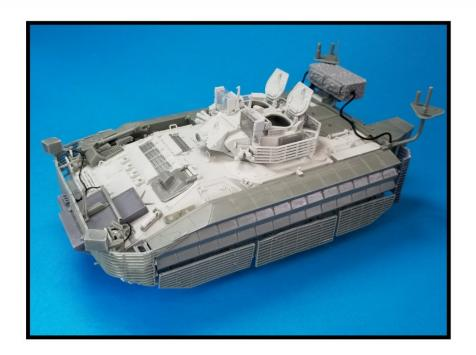
FV515 MEDIVAC vehicles were seen with both early single episcope drivers hatch and also later pattern hatch with 3 episcopes as provided in the kit.
