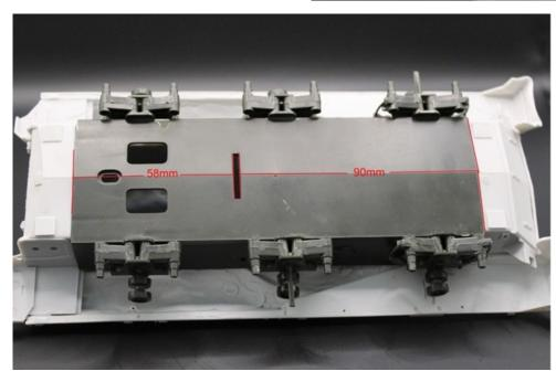
Direction for fitting to Tamiya hull.
