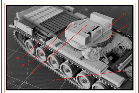
The tow-er built on Mk1 and Mk2 long hull did not have the gun rails installed.
